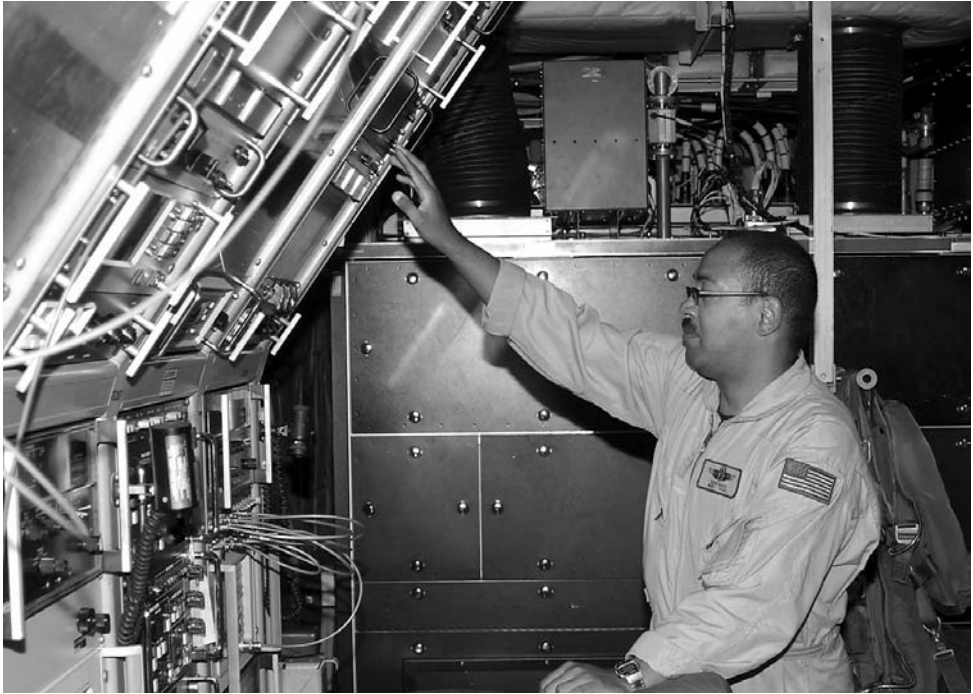
An electronic-command-system operator for EC-130 Commando Solo missions makes a final adjustment to one of his radio-frequency controls.
